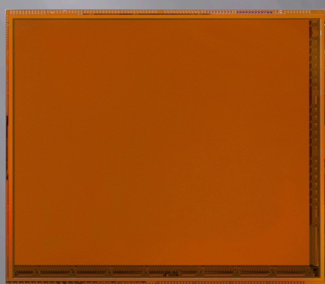
In partnership with Gatan, Inc., UCSF, and HHMI, the LBNL IC Group designed a new generation of image sensor for electron microscopy. (reticle size chip ~20mmX20mm) Process: 0.18µm CMOS.
