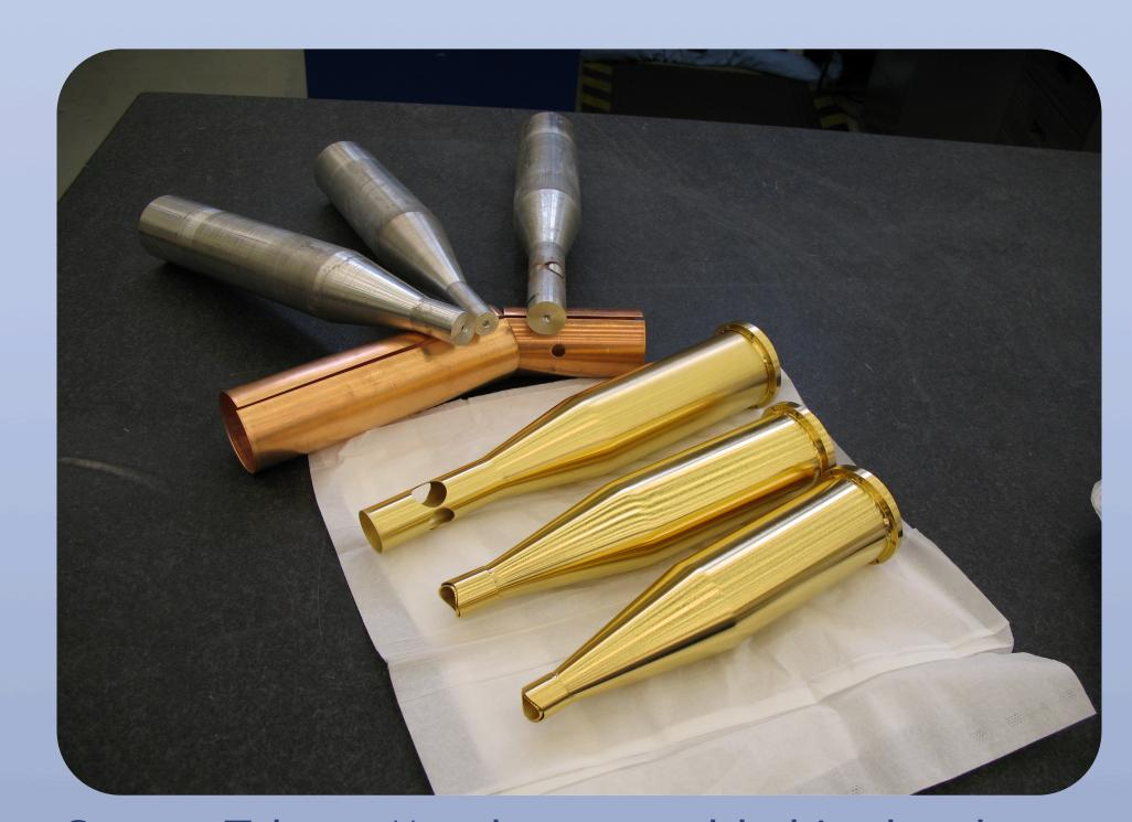
Copper Tubes - Metal spun, welded in the glove box and gold plated for a vector magnet.
