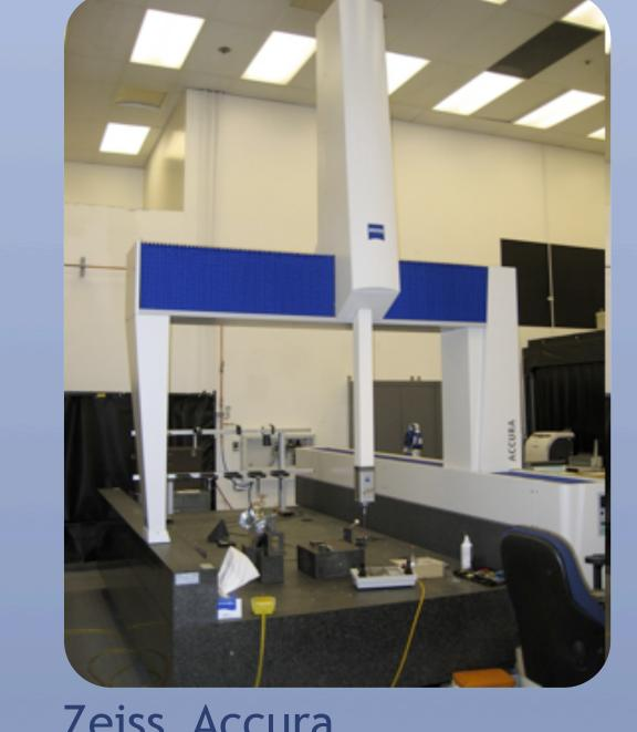
Zeiss Accura Coordinate Measuring Machine
