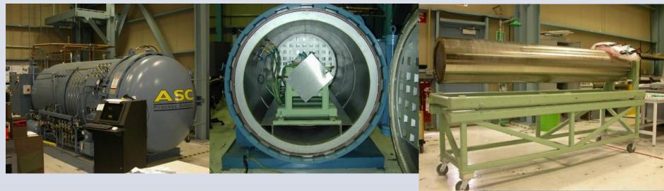
5X10 ASC Autoclave is fully automated, with integrated QC Database. Can process parts up to 1.2m X 2.7m, 150C cure temps with current pressurization system
