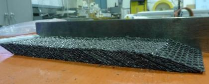
With laminates approaching the thickness of a typical bonded joint, adhesive mass is important to control for low mass structures. Resin content of custom prepregs can be tailored to allow co-cured components with no additional adhesive. For some of these low mass structures, adhesive can be 30-50% of the overall mass if not well controlled.
