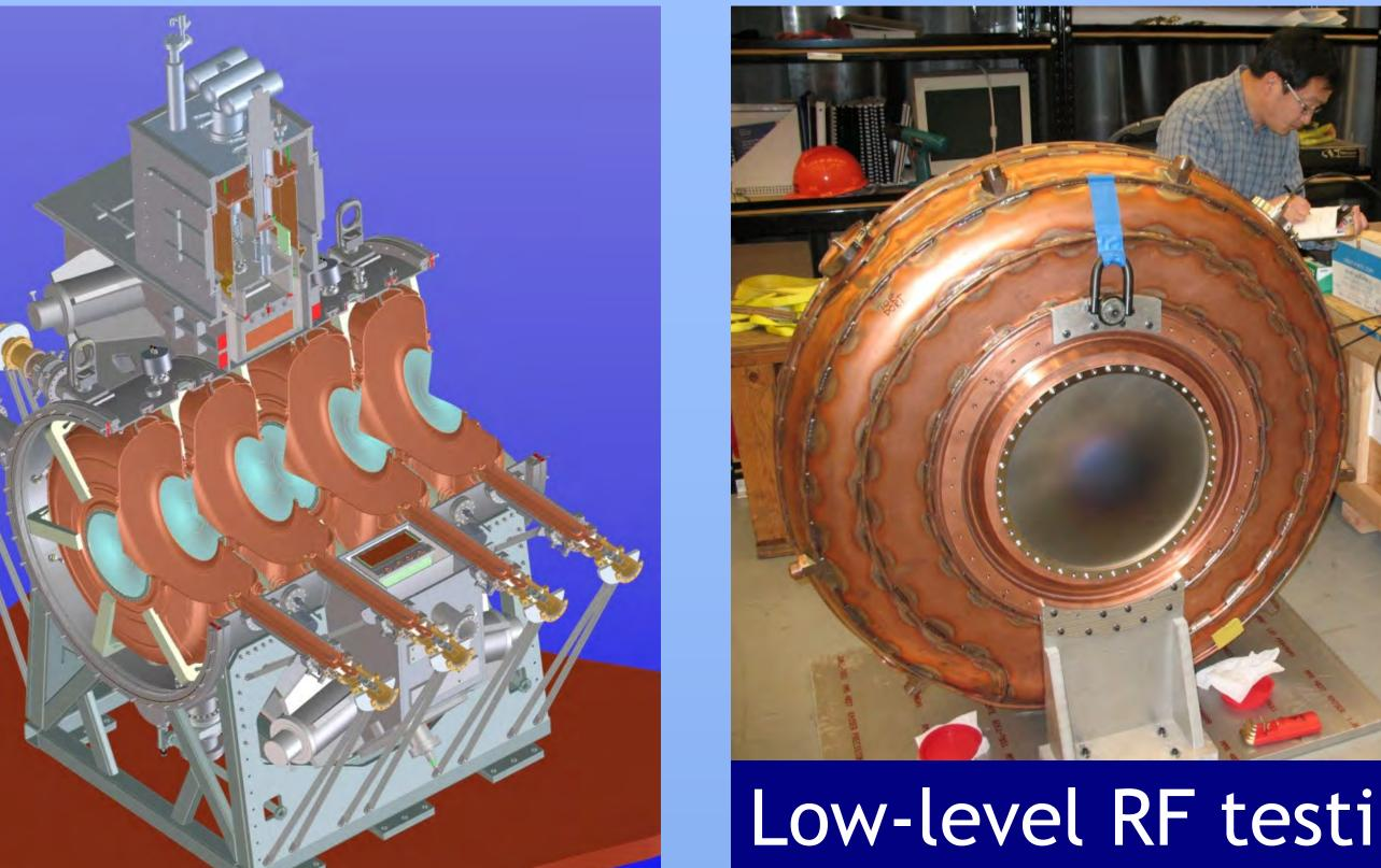
CAD model of the RFCC Modules, consisting of a superconducting coupling coil and four 201 MHz normal-conducting RF cavities
