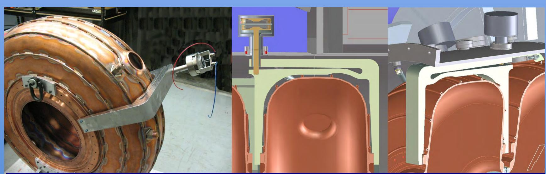
Flexure tuner designed by LBNL - 6 tuners per cavity provide a ±500 kHz range using a series of actuators
