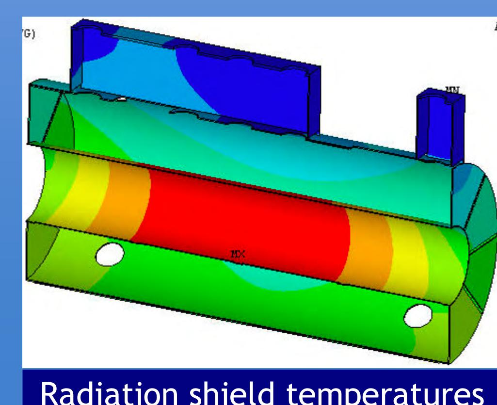
Magnet 2-D cross section Radiation shield temperatures
