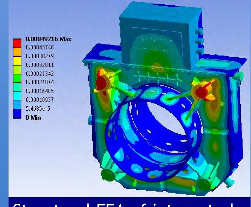
Structural FEA of integrated Cavity RF analysis Coupling Coil/vacuum vessel
